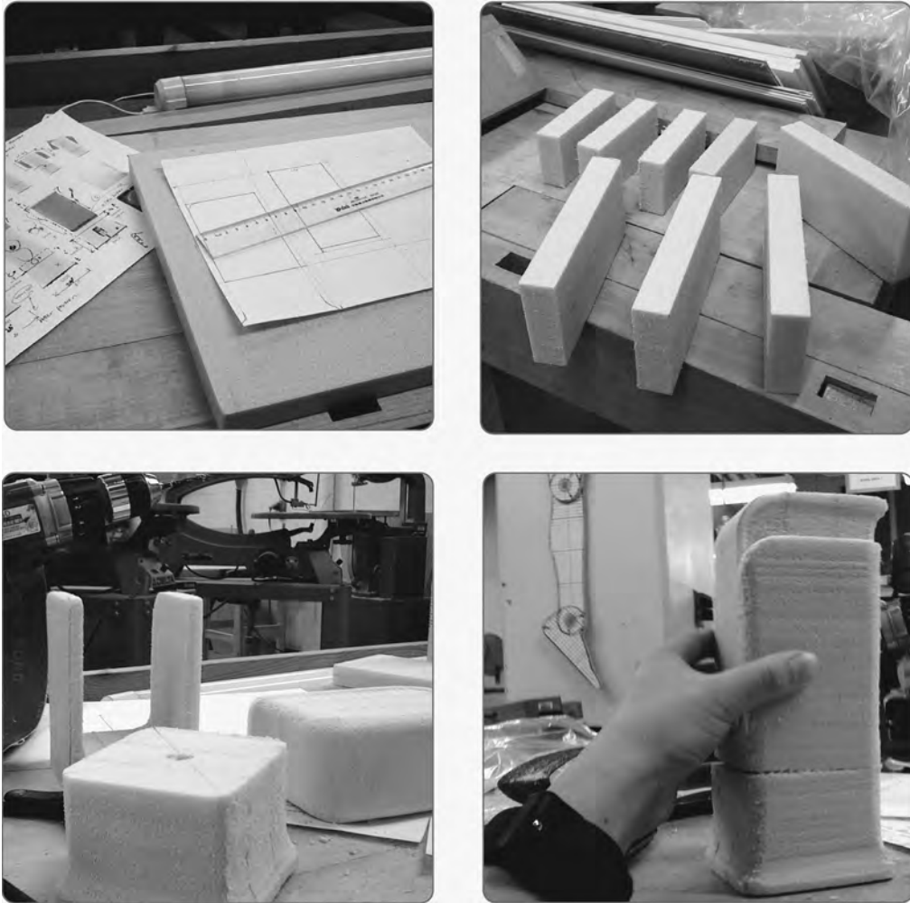
Figure 8.12 Rough conceptual models of the In-Class Communicator, a product that assists students with low vision in the activity of note-taking in the classroom (photographs and models by Liqing Zhou)
