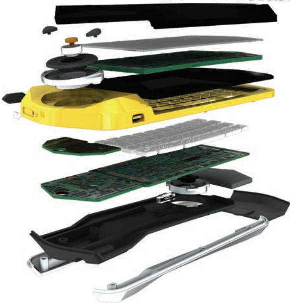
Fig. 12. A computer generated exploded view for the product Explore (image by William Atwood).
